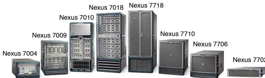
Figure 13-5 Cisco Nexus 7000 and 7700 Platform Switches
