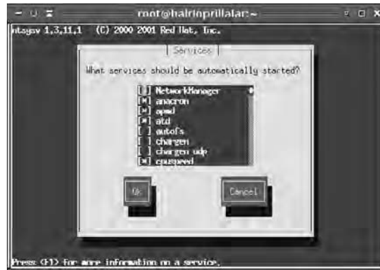
FIGURE 5.2 The ntsysv program enables you to control services from a menu of available services.
