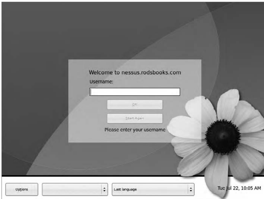
FIGURE 6.1 An XDMCP server manages local GUI logins to a Linux system.
