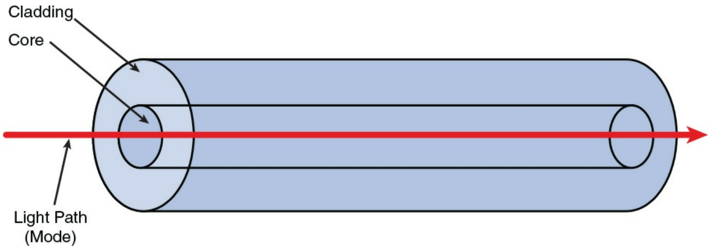
Figure 3-8 Light Propagation in Single-Mode Fiber
