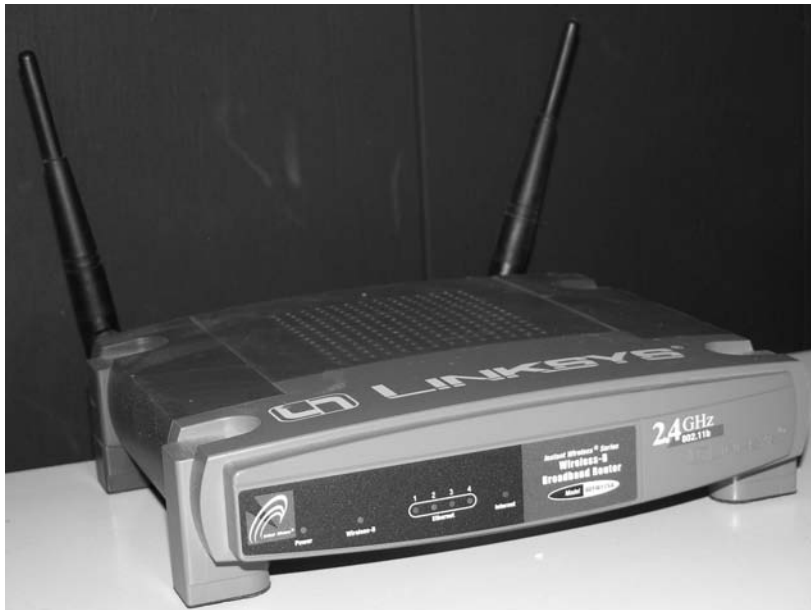
FIGURE 12.8 A wireless access point
