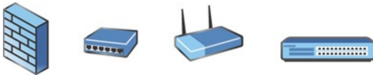
FIGURE 8.1 Diagram symbols for a firewall, a hub, a router, and a switch
