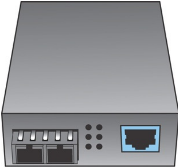
FIGURE 4.5 A common media converter
