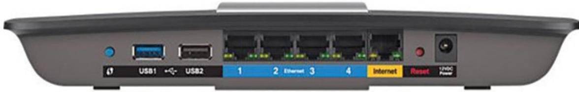
FIGURE 6.1 A wireless broadband router for a small network
